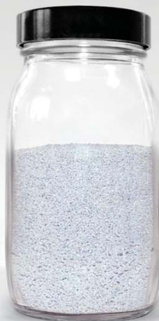
Coloured quartz (Carborundum-free particles used in Verona)
